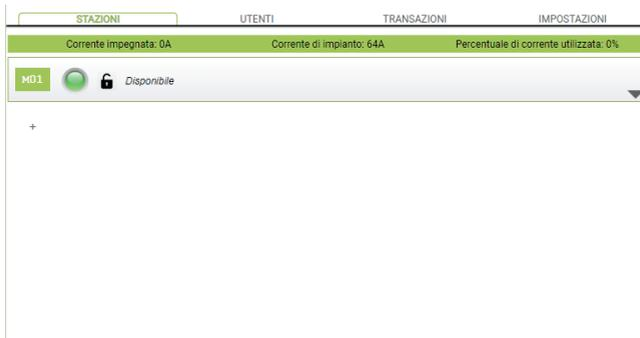
At this point it is possible to add new satellite stations, remembering that the system supports a maximum of 16 stations.
