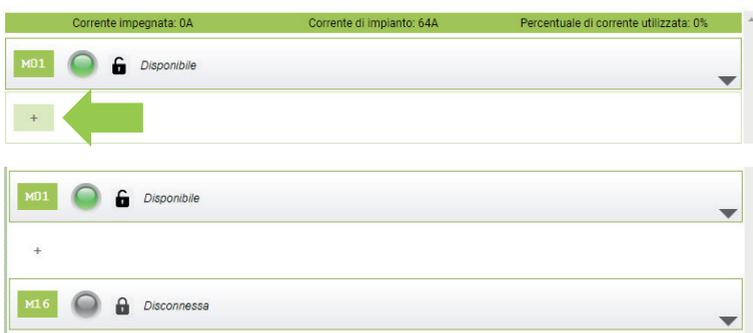
If the serial connection between the various stations has been made correctly, after a few seconds the gray status icon will turn green, which means that the station is connected correctly.
